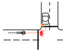
Motorist turning right does not look for wrong-way cyclist
